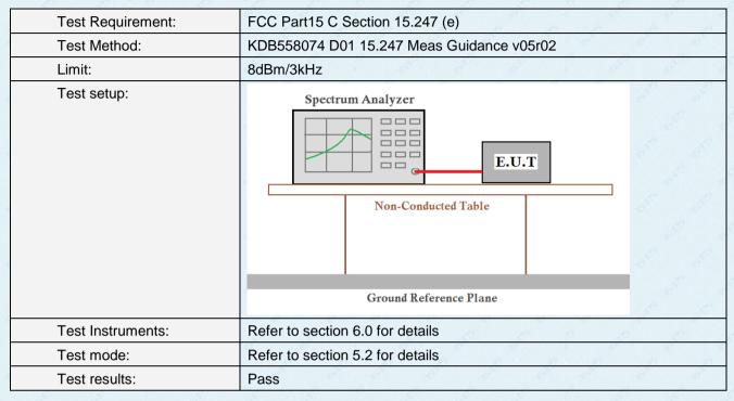
Measurement Data: The detailed test data see Appendix for WIFI 2.4G\_\_TX
