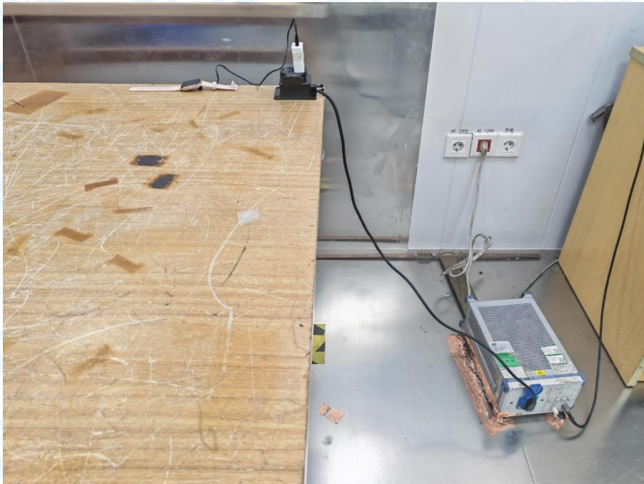
Photo of Setup for Radiated Emission (30MHz~1GHz)
