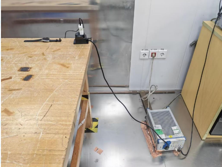
Photo of Setup for Radiated Emission (30MHz~1GHz)
