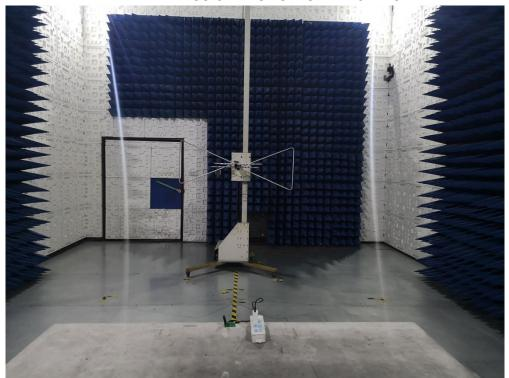
RADIATED EMISSION TEST SETUP ABOVE 1GHz
