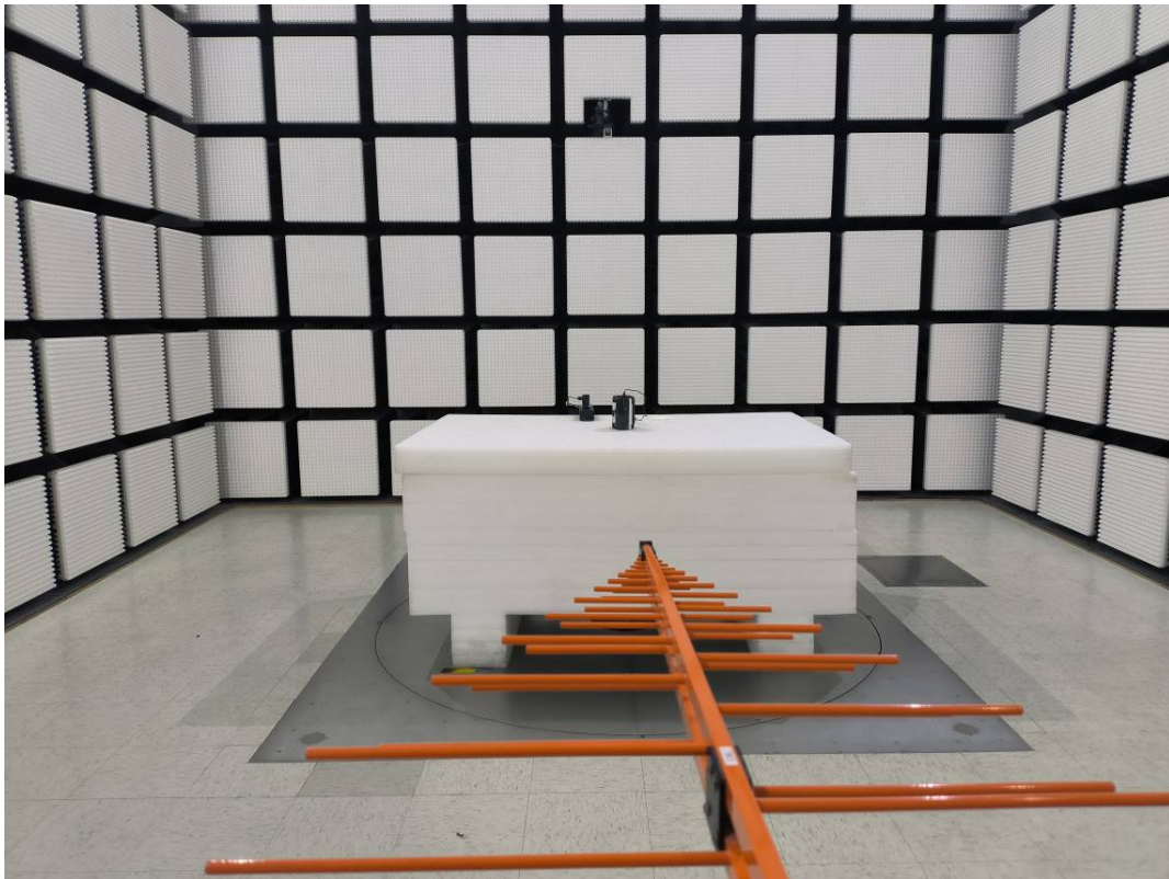
Radiated Emission 30MHz-1GHz View
