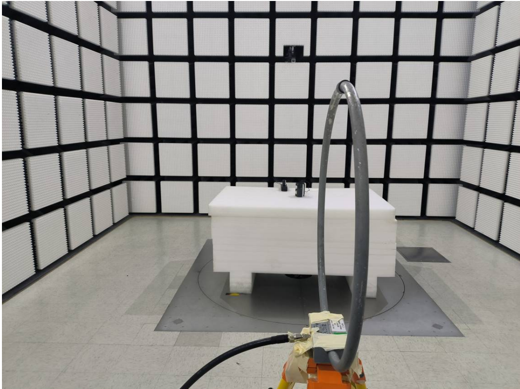
Radiated Emission 9kHz-30MHz Perpendicular View
