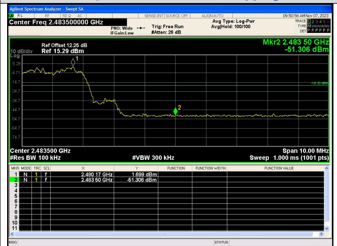
Out Of Band Emission(Right) \pi/4 DQPSK_2-DH5_Channel Hopping
