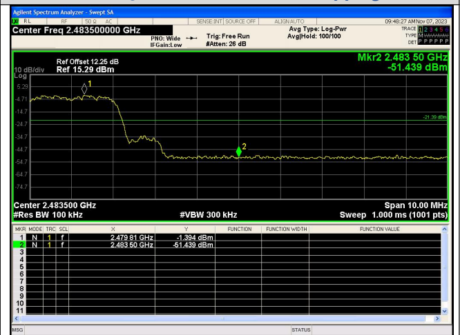
Out Of Band Emission(Right) \pi/4 DQPSK_2-DH5_Channel Hopping
