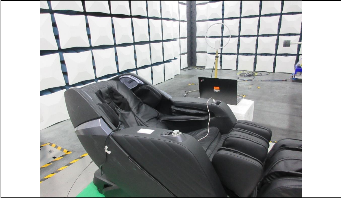
RADIATED RF MEASUREMENT SETUP (Below 30MHz)
