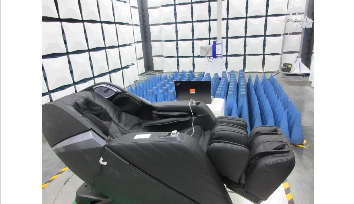
POWERLINE CONDUCTED EMISSIONS MEASUREMENT SETUP
