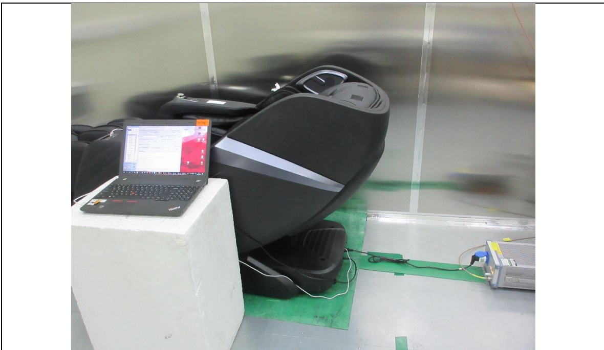
POWERLINE CONDUCTED EMISSIONS MEASUREMENT SETUP
