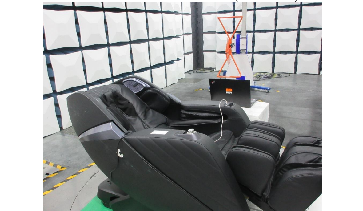
RADIATED RF MEASUREMENT SETUP (30MHz~1GHz)
