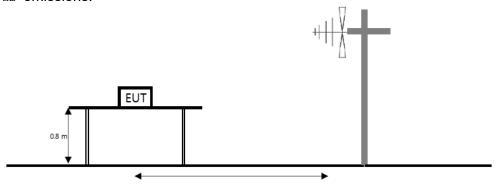
The diagram below shows the test setup that is utilized to make the measurements for emission from 1  $\mbox{ }$  to the tenth harmonic of the highest fundamental frequency or to 40  $\mbox{ }$  emissions, whichever is lower.
