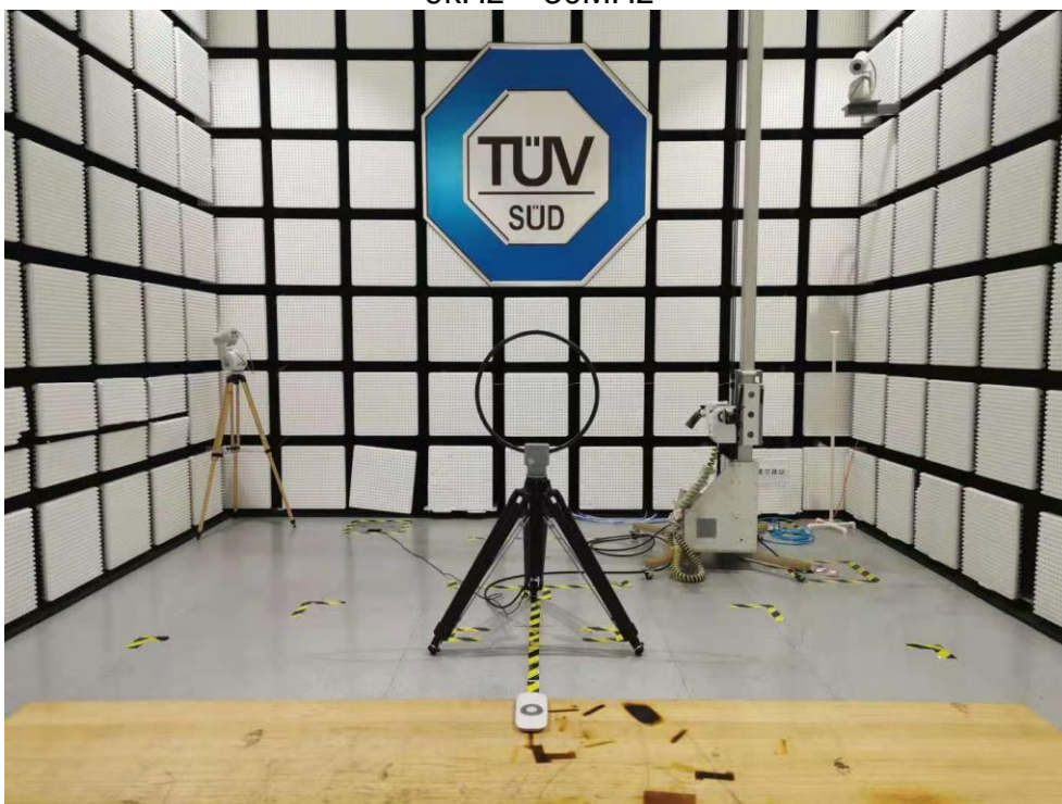
Radiated Emission Setup 9kHz ~ 30MHz
