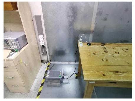
Radiated Spurious Emissions Test Frequency From 30MHz-1000MHz
