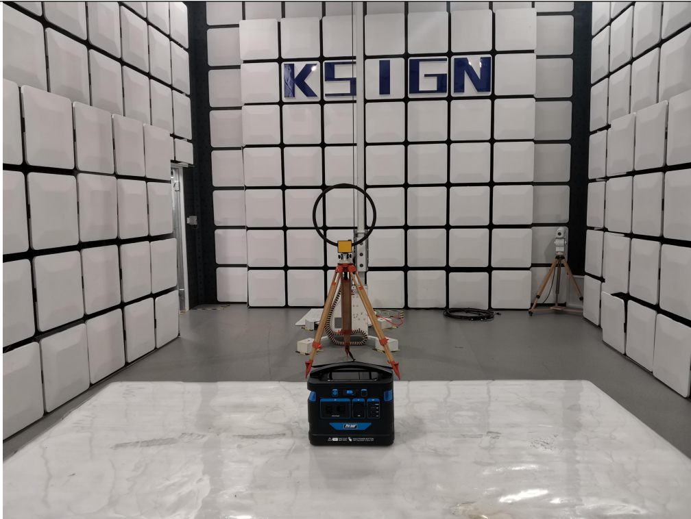
RADIATED EMISSION TEST SETUP(30MHz-1GHz)
