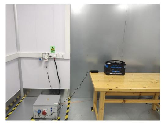
RADIATED EMISSION TEST SETUP 9KHz-30MHz
