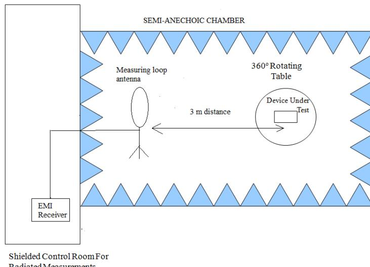
Radiated measurements setup 30 MHz to 200 MHz:
