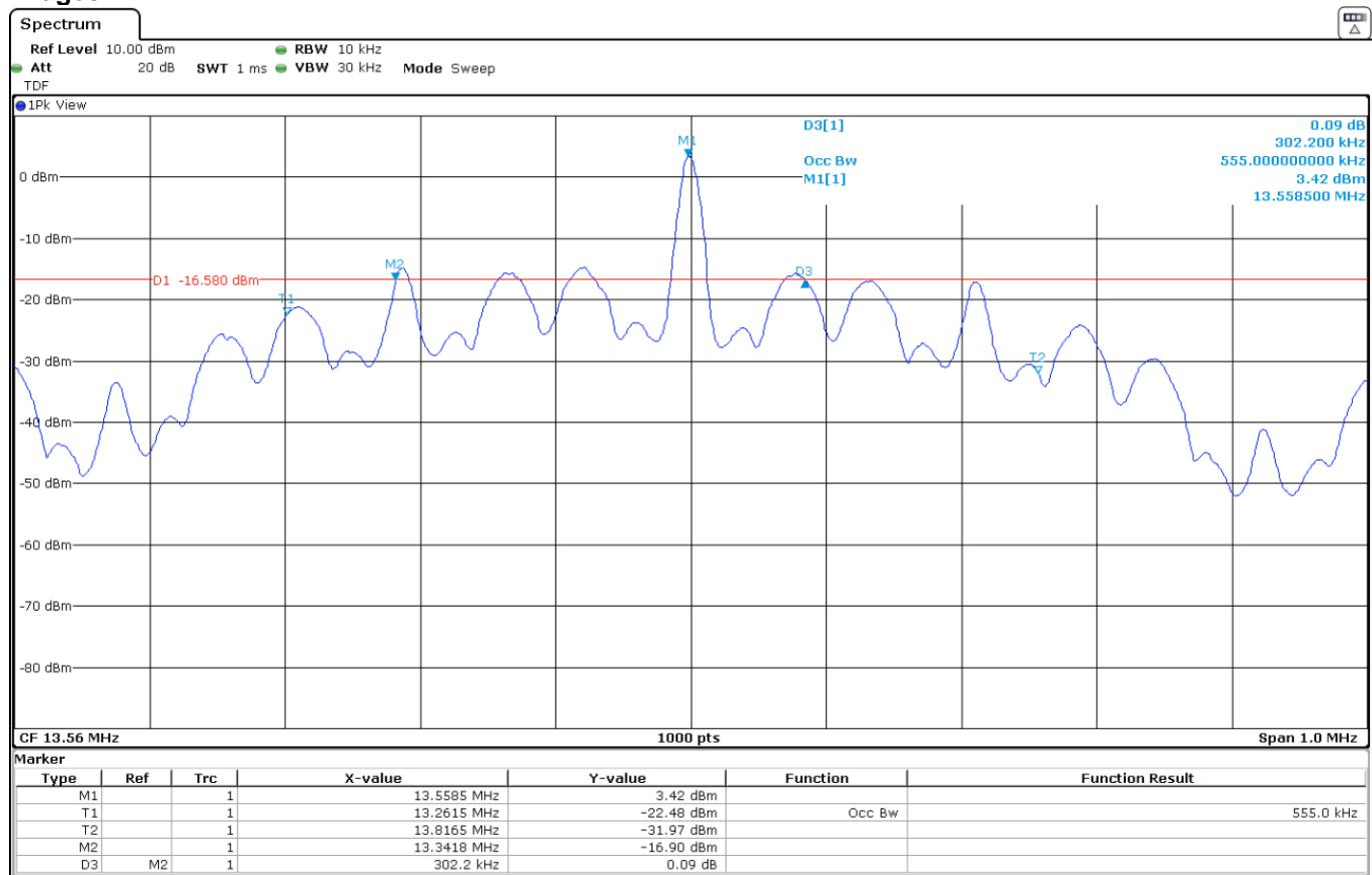
**FCC 15.225 (a) (b) (c) / RSS-210 B.6 (a) (b) (c). Field strength of emissions within the band 13.553 -13.567 MHz, 13.410 - 13.553 MHz and 13.567 - 13.710 MHz, 13.110 - 13.410 MHz and 13.710 - 14.010 MHz**
