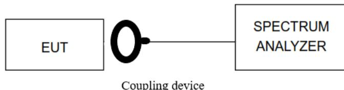
For extreme test conditions the EUT was placed inside a climatic chamber and connected to a spectrum analyzer using a low-loss cable and a coupling device. An external DC power supply was connected to the EUT for voltage variation test.
