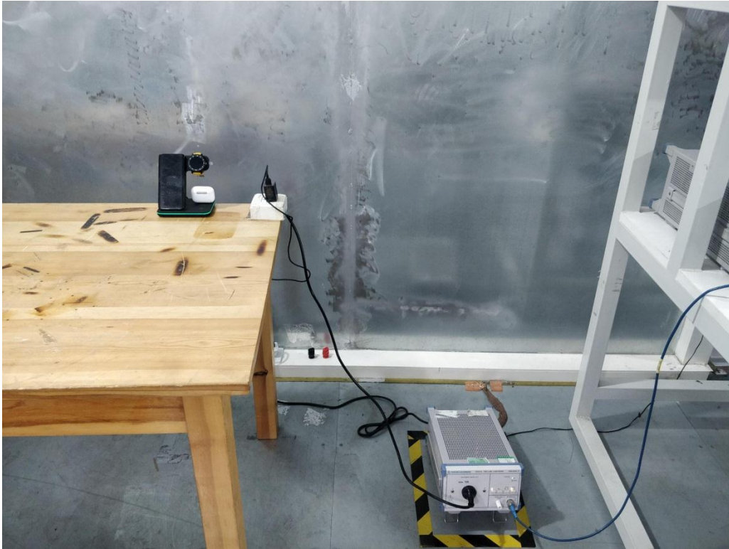
Conducted Emission-AC adapter charge mode
