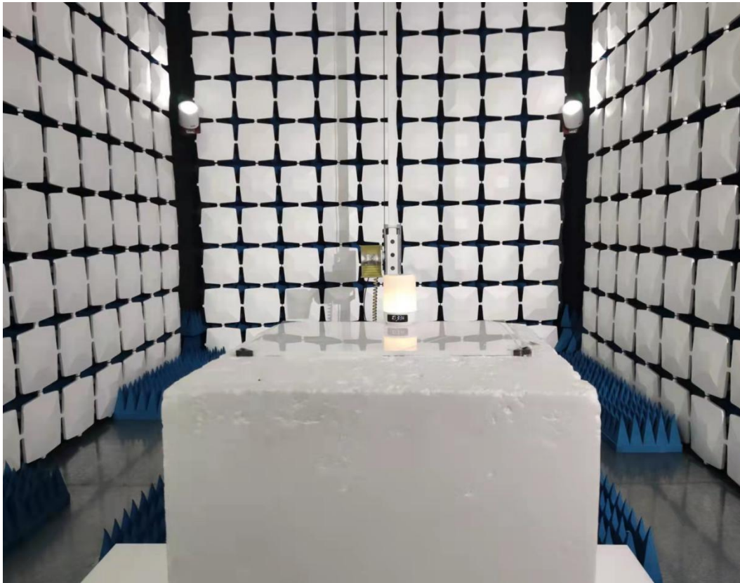
Below 1GHz for radiated emission test setup
