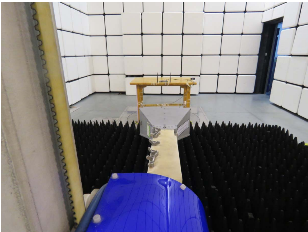
Picture 2: Radiated Spurious Emissions Test setup
