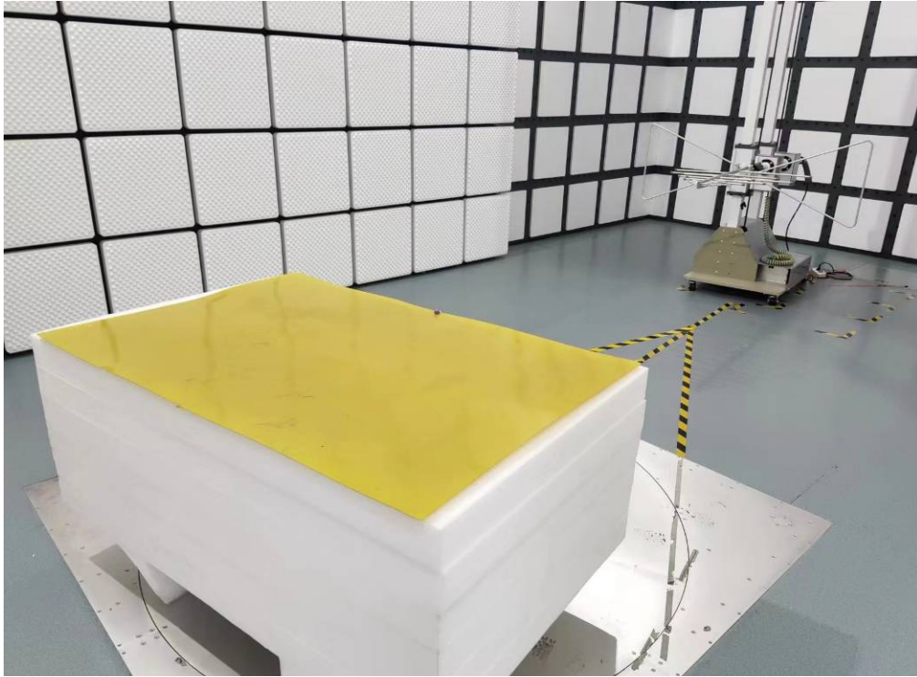
Photo of Radiated Emission Measurement (Above 1G)
