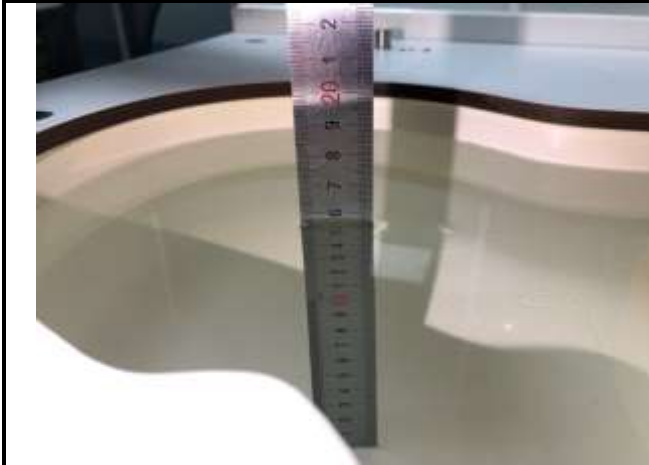
Fig. 9.7 Photo of Liquid Height for Head SAR (5200MHz~5800MHz) (depth>15cm)
