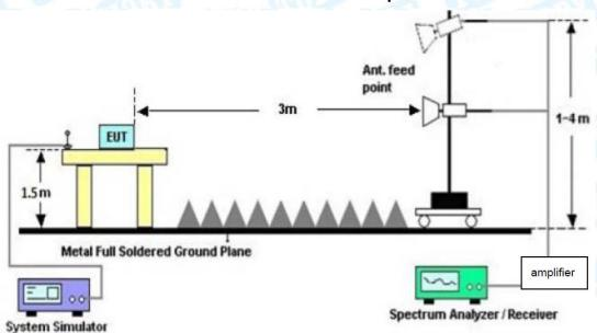
**Above 1GHz Test Setup**
