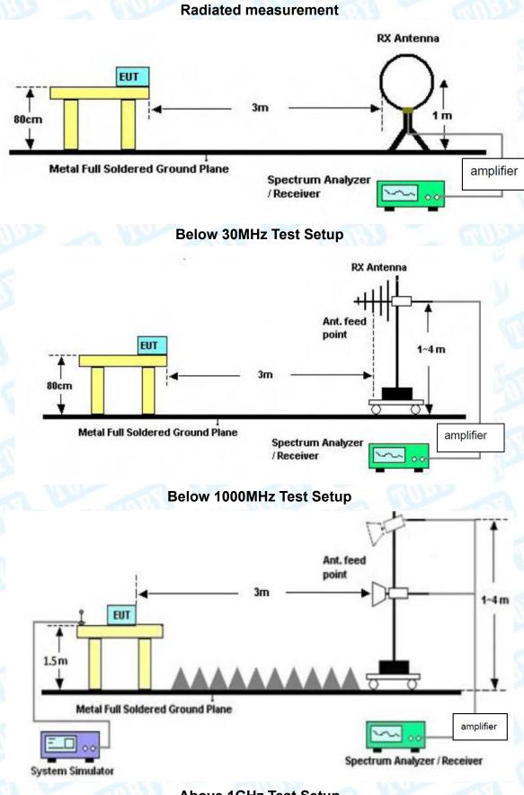
Above 1GHz Test Setup
