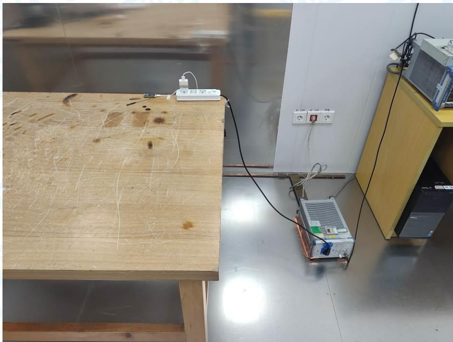
Photo of Setup for Conducted Emission
