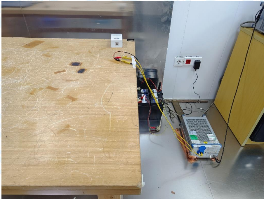
Photo of Setup for Conducted Emission
