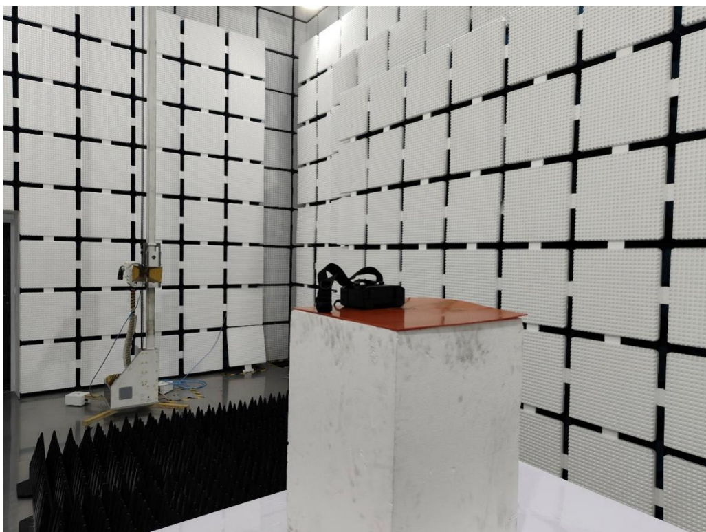
Photograph 2: Set-up photo for Radiated Spurious Emission, above 1GHz
