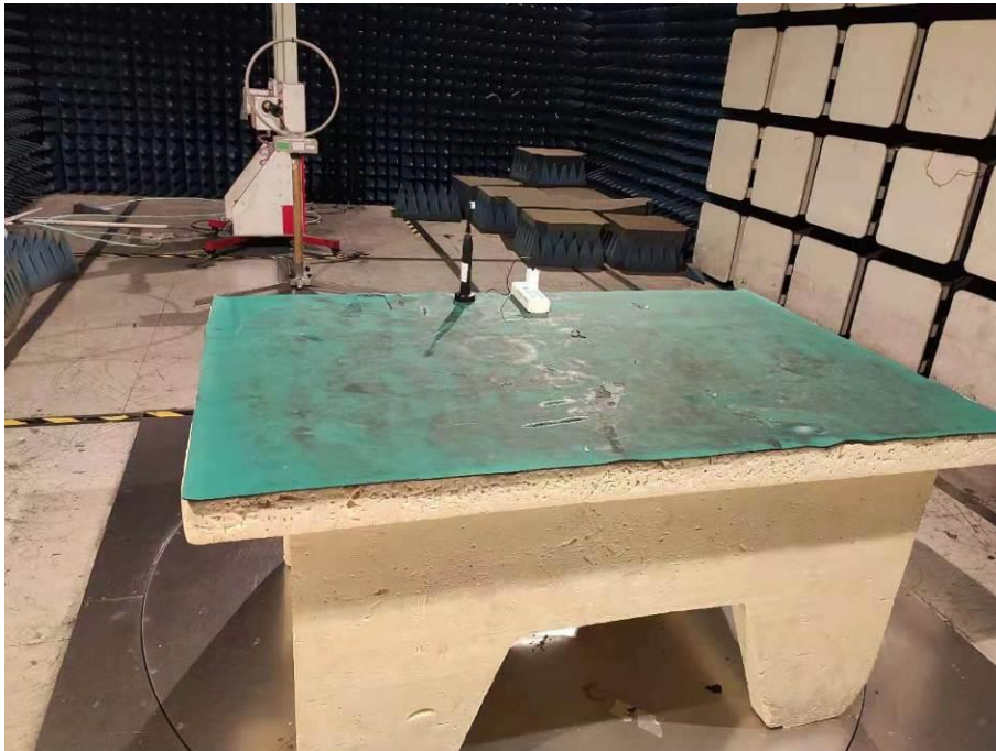
Spurious Emission Test Setup (Below 30MHz)
