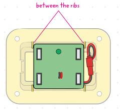
The switch and wires will be loose. Make sure that they tuck down on the sides of the yellow ribs, not above them. 3
