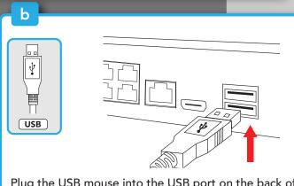
Plug the USB mouse into the USB port on the back of the NVR.
