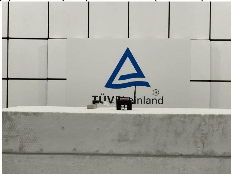
Photograph 2: Test Setup for Spurious Emissions (Front View 2)
