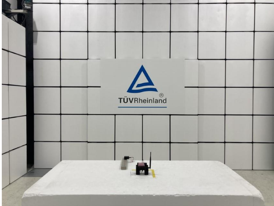
Photograph 2: Test Setup for Spurious Emissions (Front View 2)
