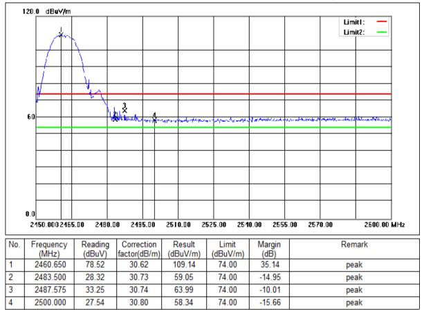
Mode:a; Polarization:Horizontal; Modulation:b; bandwidth:20MHz; Channel:High
