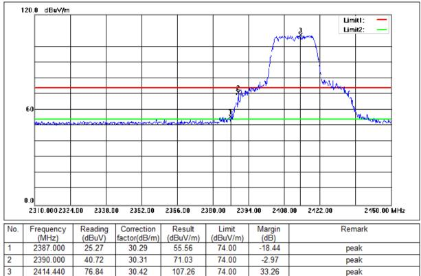
Mode:a; Polarization:Horizontal; Modulation:g; bandwidth:20MHz; Channel:Low
