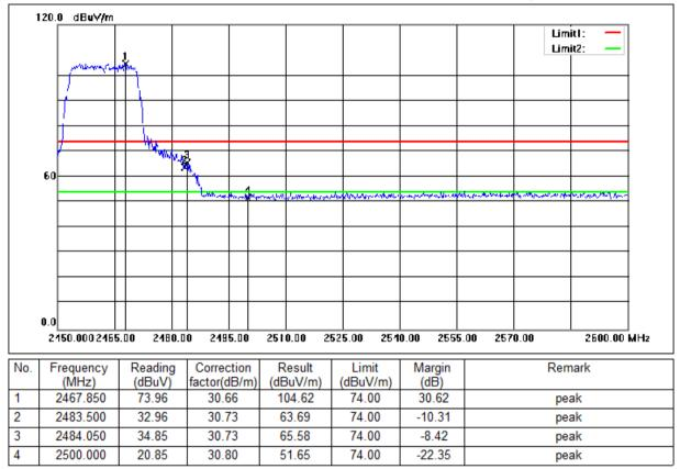
Mode:a; Polarization:Horizontal; Modulation:n; bandwidth:20MHz; Channel:High
