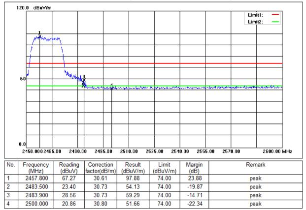
Mode:a; Polarization:Vertical; Modulation:g; bandwidth:20MHz; Channel:High
