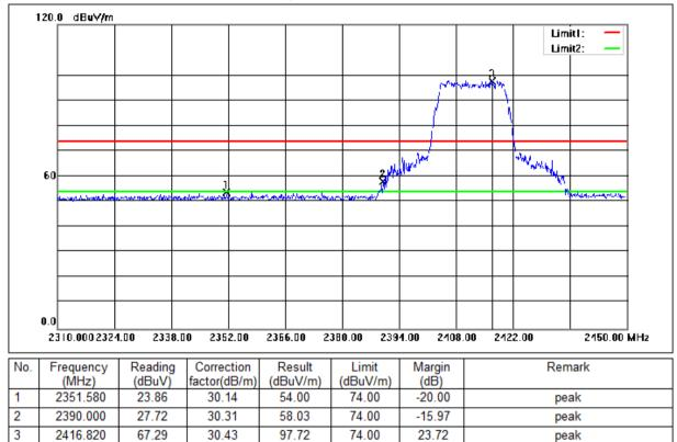
Mode:a; Polarization:Vertical; Modulation:g; bandwidth:20MHz; Channel:Low
