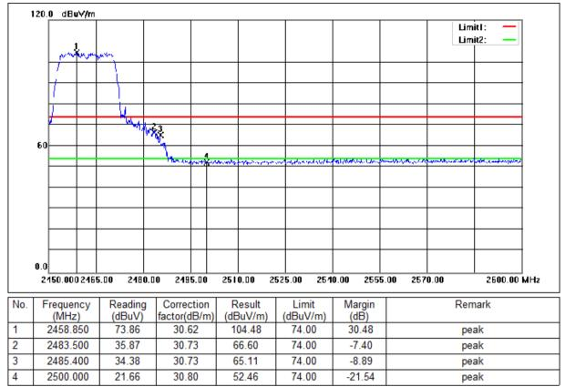
Mode:a; Polarization:Vertical; Modulation:n; bandwidth:20MHz; Channel:High
