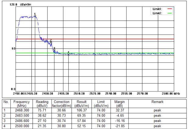
Mode:a; Polarization:Horizontal; Modulation:g; bandwidth:20MHz; Channel:High
