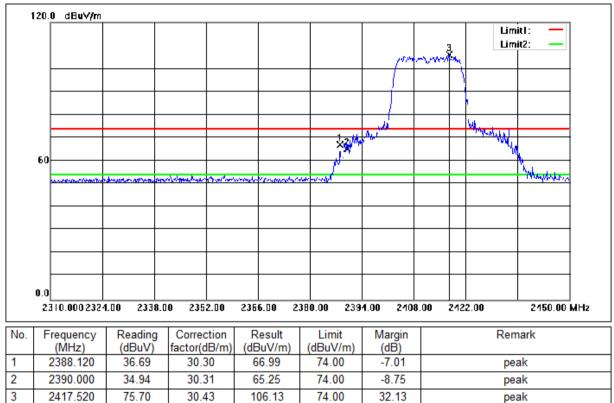
Mode:a; Polarization:Horizontal; Modulation:n; bandwidth:20MHz; Channel:Low
