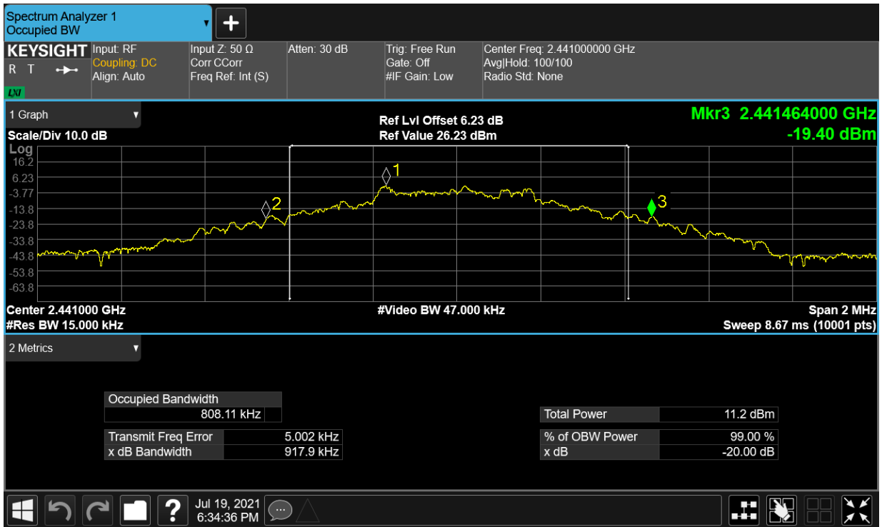
-20dB Bandwidth NVNT 1-DH1 2480MHz Ant1
