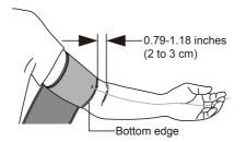
Make sure that the air tube is positioned on the inside of your arm and wrap the cuff securely, so it can not move around your arm.
