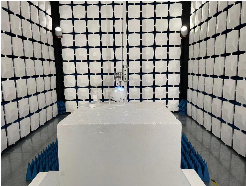
Above 1GHz for radiated emission test setup
