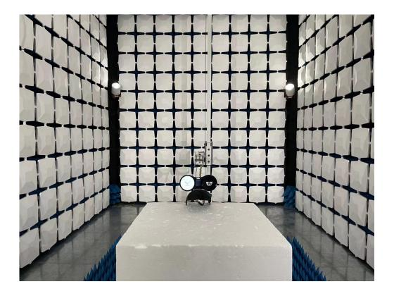
Blow 1GHz for radiated emission test setup
