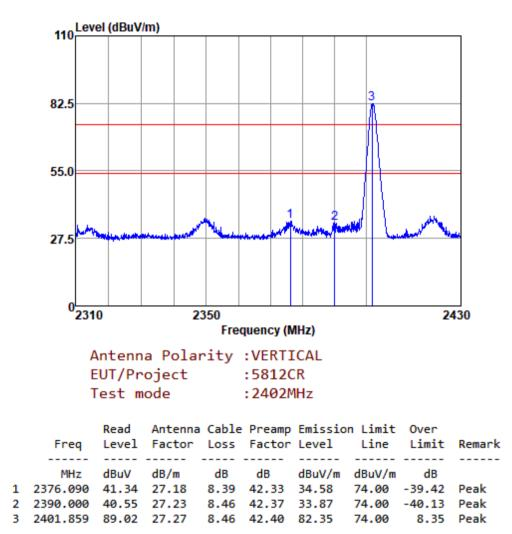
Mode:c; Polarization:Vertical; Modulation:GFSK; ; Channel:Low (1M)
