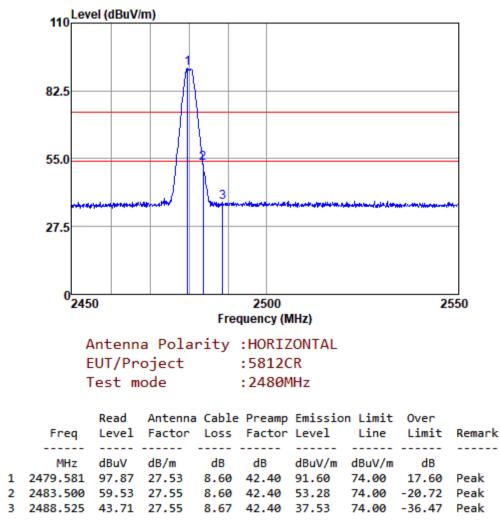
Note:Emission Level=Read Level+Antenna Factor+Cable loss-Preamp Factor
