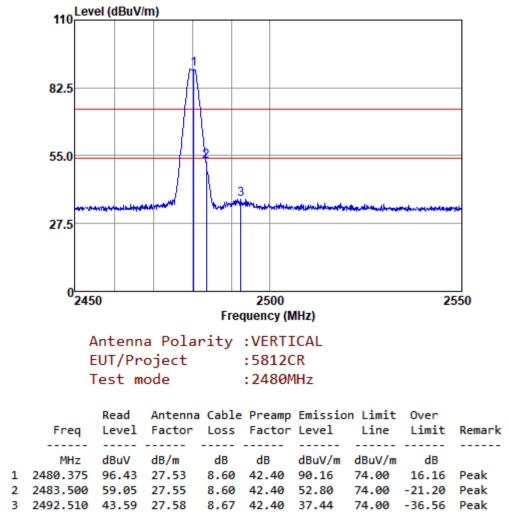
Note:Emission Level=Read Level+Antenna Factor+Cable loss-Preamp Factor
