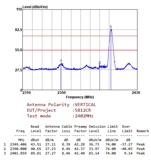
Note:Emission Level=Read Level+Antenna Factor+Cable loss-Preamp Factor
