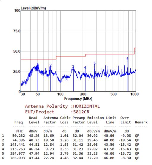
Note:Emission Level=Read Level+Antenna Factor+Cable loss-Preamp Factor
