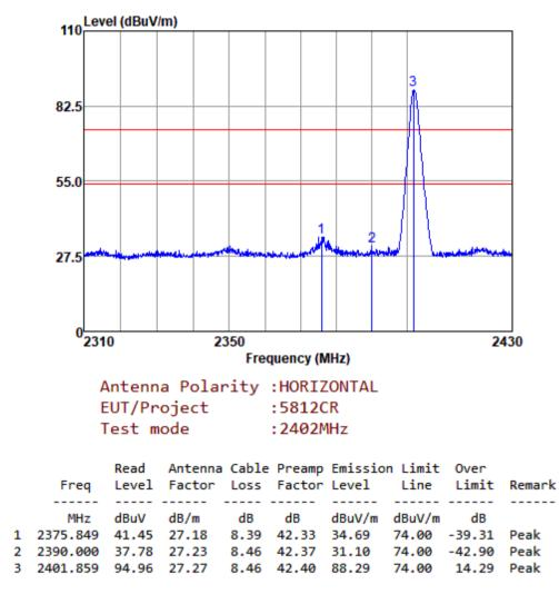
Note:Emission Level=Read Level+Antenna Factor+Cable loss-Preamp Factor
