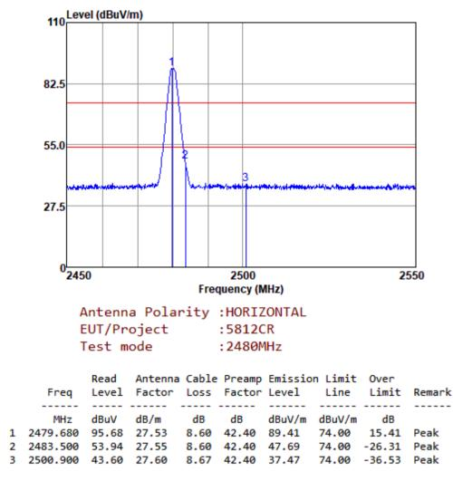
Note:Emission Level=Read Level+Antenna Factor+Cable loss-Preamp Factor
