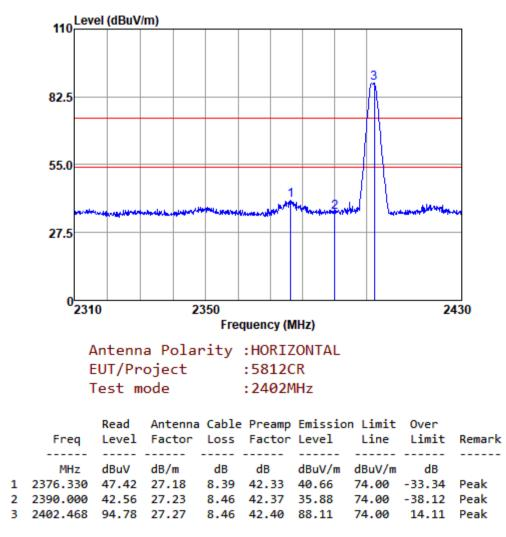
Note:Emission Level=Read Level+Antenna Factor+Cable loss-Preamp Factor
