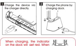
on the dock will get red. When fully charged, It will turn green. if the phone is not placed if the phone is not placed properly with the dock, the indicator will display green, please reposition the phone until it is well placed.
