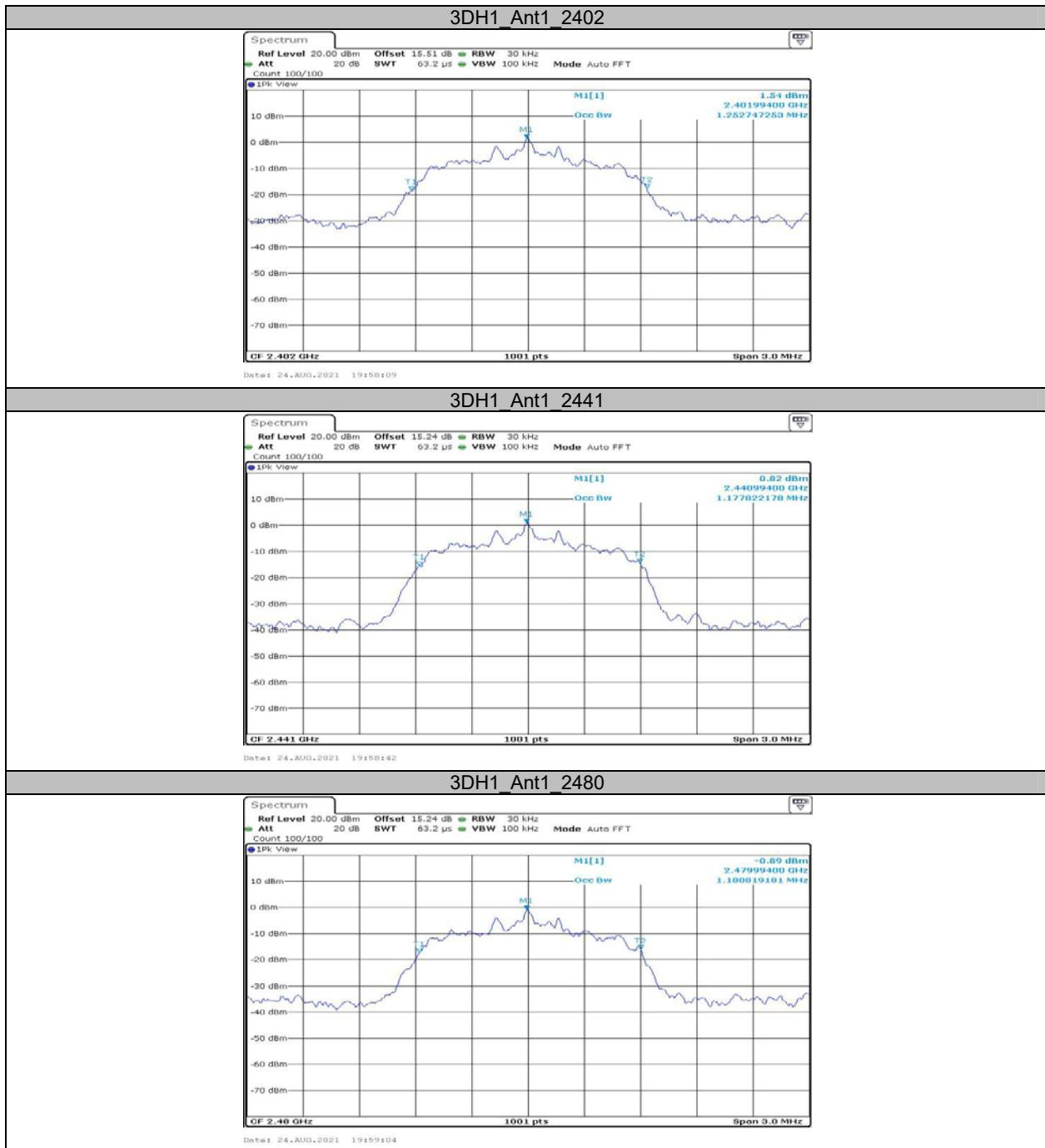
**Appendix C: Maximum conducted Peak output power****Test Result**
