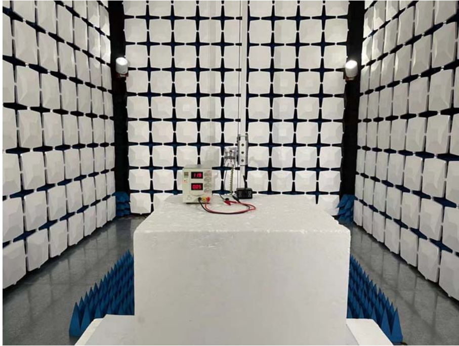
Above 1GHz for radiated emission test setup
