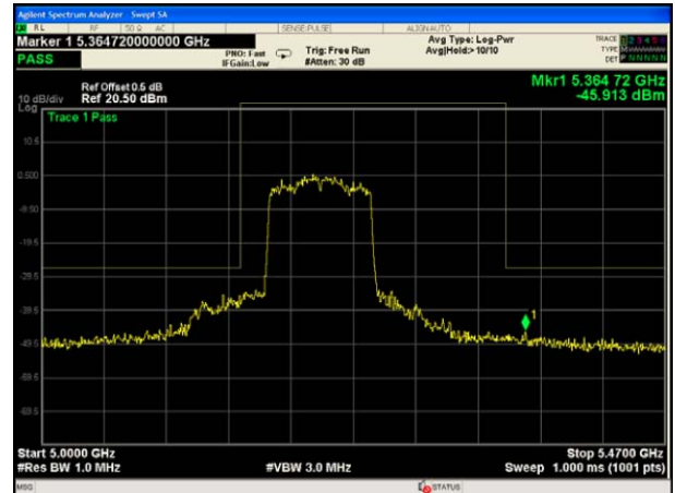
802.11 ac(HT80)UNII-1 Band edge-right side
