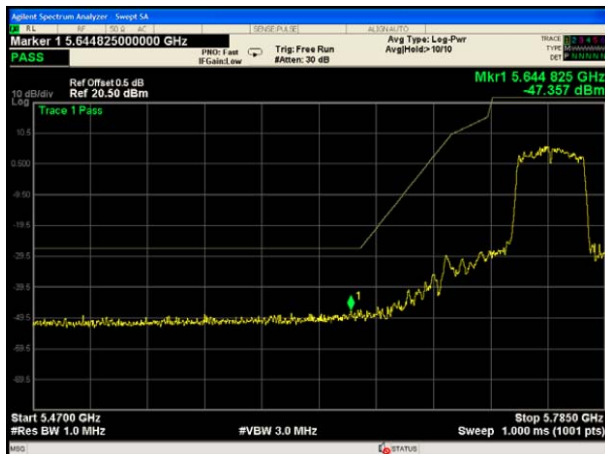
802.11ac(HT40)UNII-3 Band edge-left side
