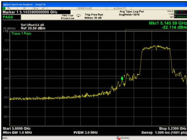
802.11 ac(HT40)UNII-1 Band edge-left side
