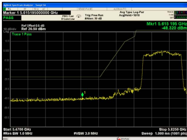
802.11ac(HT80)UNII-3 Band edge-left side
