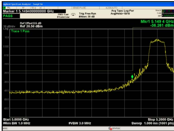
802.11 ac(HT20)UNII-1 Band edge-left side
