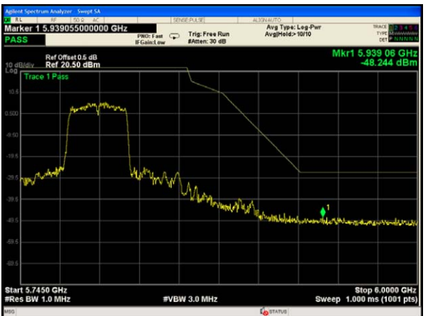
802.11 ac (HT40)UNII-3 Band edge- right side
