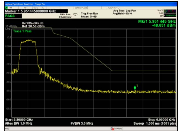
802.11 ac (HT20)UNII-3 Band edge- right side
