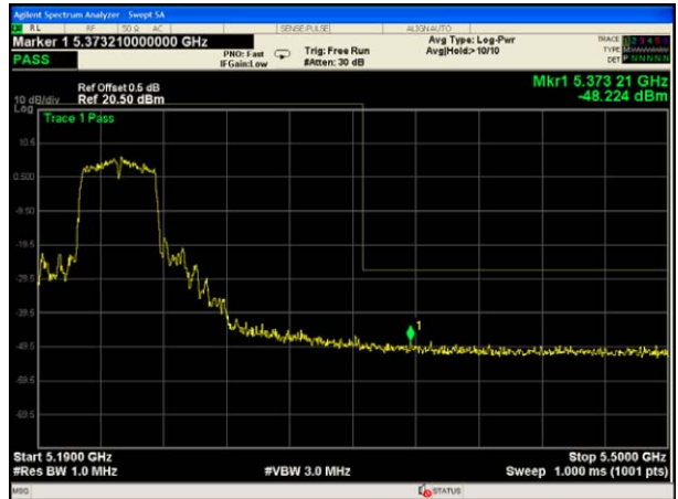
802.11 ac(HT40)UNII-1 Band edge-right side
