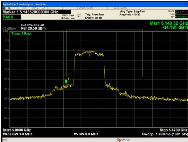
802.11 ac(HT80)UNII-1 Band edge-left side
