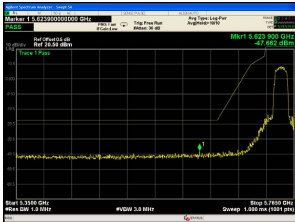
802.11ac(HT20)UNII-3 Band edge-left side
