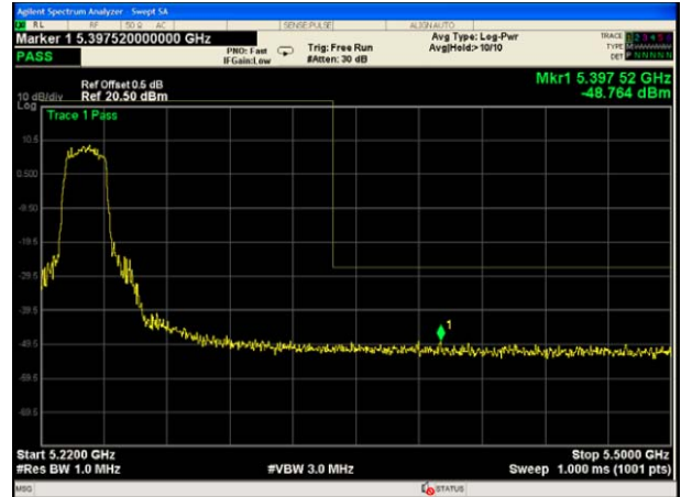
802.11 ac(HT20)UNII-1 Band edge-right side
