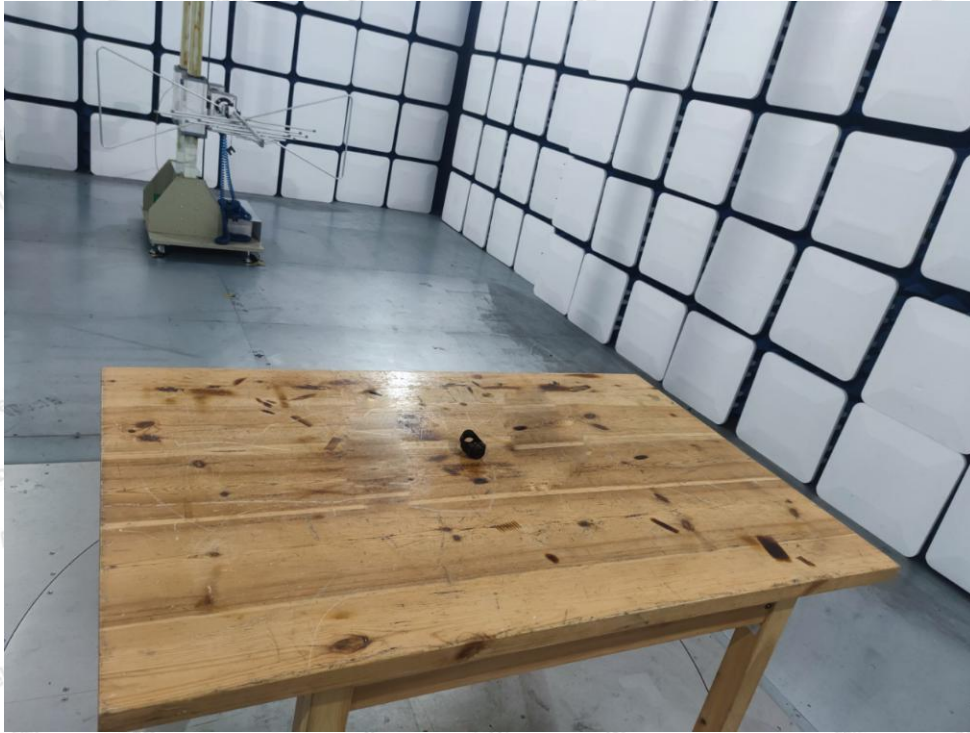
Photo of Radiation Emission Test
