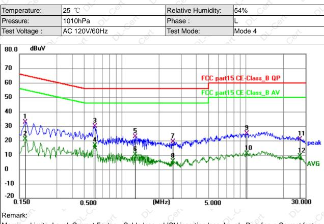
Margin = Limit – Level, Correct Factor = Cable lose + LISN insertion loss, Level= Reading + Correct factor
