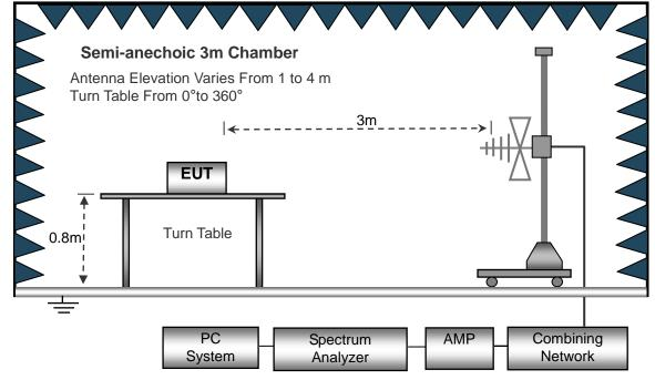
(C) Radiated Emission Test-Up Frequency Above 1GHz
