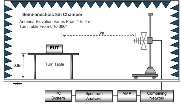
(C) Radiated Emission Test-Up Frequency Above 1GHz
