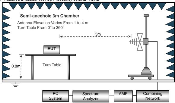
(C) Radiated Emission Test-Up Frequency Above 1GHz
