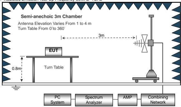
(C) Radiated Emission Test-Up Frequency Above 1GHz
