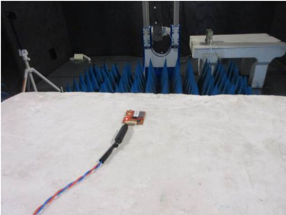
TEST SETUP PHOTO(S) RADIATED EMISSIONS – POSITION 1
