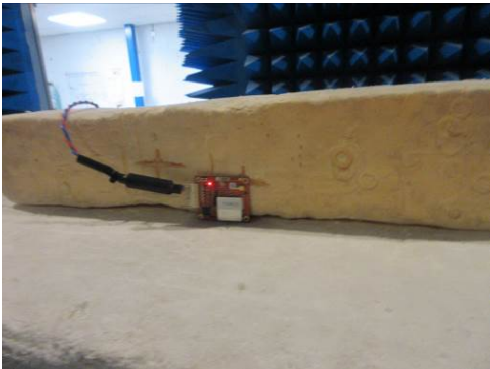
TEST SETUP PHOTO(S) RADIATED EMISSIONS – POSITION 2
