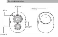
Specifications MODELIShutter Communication Bluetooth Version, 3.0 Transmit frequency 2.402GHz -2.480GHz Communication distance 10m(30ft) Battery life CR2032 X1 cell/about 6 months Dimension 48mm X 30mm X 10mm Weight About 8a
