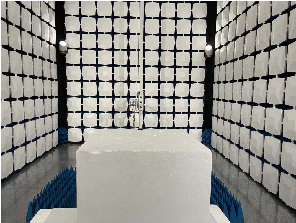
Above 1GHz for radiated emission test setup
