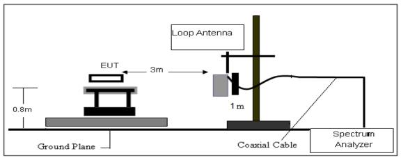
(B) Radiated Emission Test-Up Frequency 30MHz~1GHz
