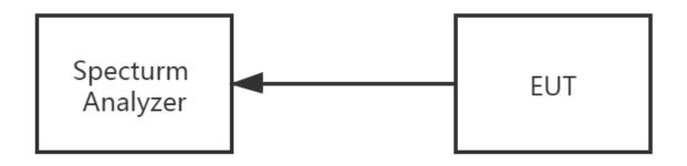
The EUT which is powered by the \${ POWER BY}, is connected to the Spectrum Analyzer; the RF load attached to the EUT antenna terminal is 50 Ohm; the path loss as the factor is calibrated to correct the reading. Make the measurement with the spectrum analyzer's resolution bandwidth(RBW) = 100 kHz. In order to make an accurate measurement, set the span greater than RBW.
