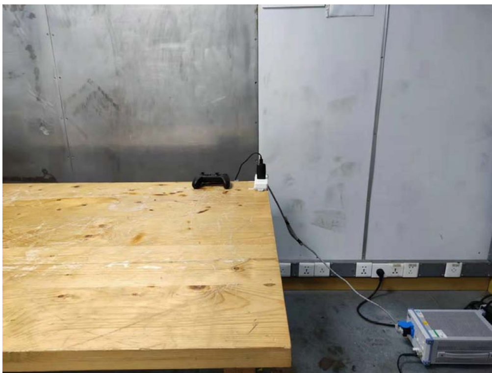
Photo of Conducted Emission Measurement
