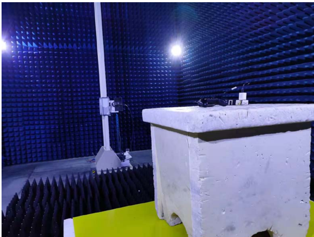
Photo of Radiated Emission Measurement Above 1GHz
