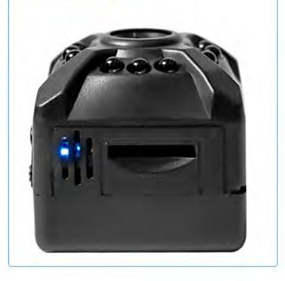
Step 2:Charge the camera by the supplied cable, then turn on the camera. When blue light on,press "Reset"button about 5 seconds,if blue light flashes, reset is successful.
