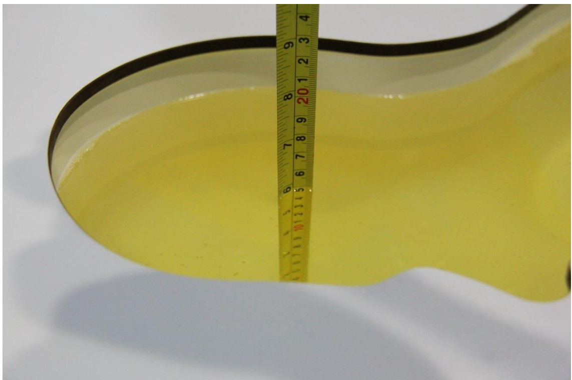
Picture 7-4 Liquid depth in the Head Phantom (2300MHz)
